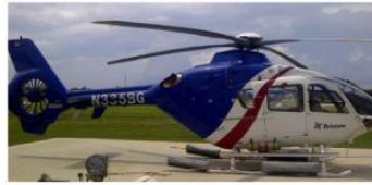
Light Twin Engine: 6-7 passengers, 350 mile range, 135 knots
