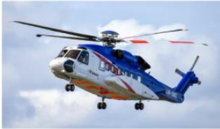
Heavy Twin Engine: 16-19 passengers, 500 mile range, 145 knots
