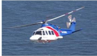
Medium Twin Engine: 12 passengers, 350 mile range, 145 knots
