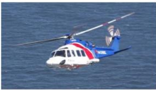
Medium Twin Engine: 12 passengers, 450 mile range, 145 knots
