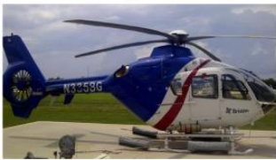
Light Twin Engine: 6-7 passengers, 325 mile range, 130 knots
