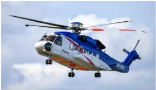
Heavy Twin Engine: 16-19 passengers, 500 mile range, 145 knots
